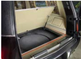
Rear under-floor storage compartment with hinged lid and spare tire storage sump. Item #Y316
